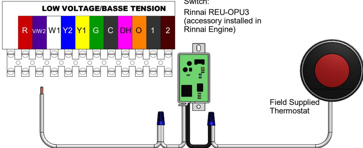
*Connections to the Air Handler PC Board.
